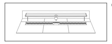
6 Lower the channel insert into the channel cut-out and allow to cure.
