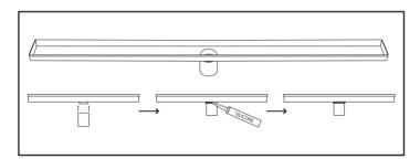
Attach a stainless steel spigot to the channel and lock in position. Create a water-tight seal with silicone sealant and allow to cure.
