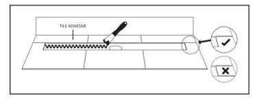
**5** Apply an appropriate amount of tile adhesive or silicon to the channel cut-out.
