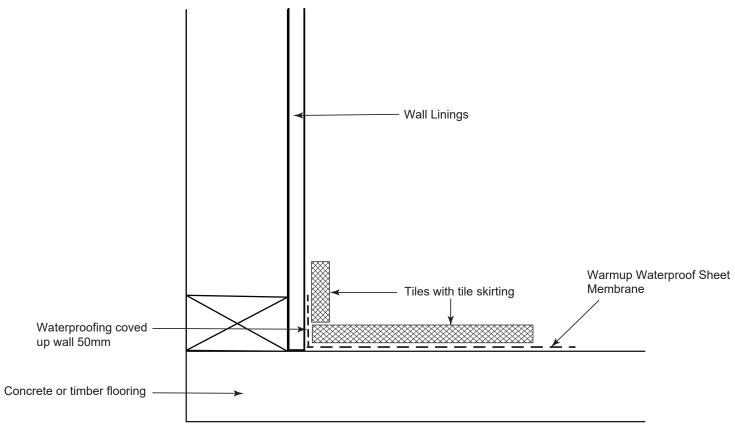
Note: If using 6mm Marmox Insulation Board, this is installed on top of the waterproofing.
